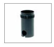
For mounting Outdoor Microphones G.R.A.S. 41AM/41CN (fitted with Pole Adapter AM0029) on a tripod. Has 1/2" RG (ISO 228/1) male thread on top and 3/8" UNC-16 female thread at the bottom.
