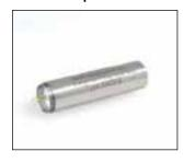
The RA0016 is a 20 dB attenuator for inserting between a 1/2" microphone and preamplifier. It will attenuate the output signal of the microphone by 20 dB in order to avoid overloading the preamplifier or following analyzer.
