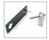
For checking the AEN and REF speaking positions on the Telephone Test Head G.R.A.S. 45AA.
