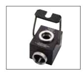
A larger-volume Coupler for enabling Pistonphone G.R.A.S. 42AA and 42AP to produce a sound pressure level of 94 dB instead of 114 dB re. 20 µPa. Essential when calibrating highly sensitive, G.R.A.S. Lownoise Measuring
