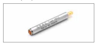
CCP preamplifier with integrated SMB connector. For use with 1/4" prepolarized microphones. For direct use on G.R.A.S. Array Modules PR0001 and PR0002 connected to constant-current input devices. Includes built-in TEDS which enables it to be programmed as a complete unit together with a microphone.
