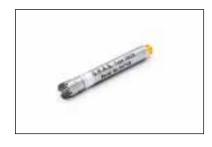
46BE is a 1/4" freefield microphone set with low sensitivity for high level and high frequency measurements; with built-in TEDS and Microdot connector.
