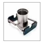
Two-port high pressure coupler for 1/2" microphones. Used in comparison calibrations between two 1/2" microphones; one of which is a reference microphone. It can also be used in measuring the P-I (Pressure-Intensity) Index of intensity probes at 250 Hz. For use with Pistonphone G.R.A.S. 42AC.
