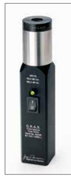
microphones. It complies with the requirements of IEC 60942 (1988) Class 1 and is PTB approved.
