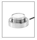
The microphone set 47AX is a low profile 1/2" precision pressure microphone with built-in CCP preamplifier. With a height (to the diaphragm) of only 8 mm, 47AX is suitably designed for flush mounting in plates in ground array applications and other applications with size constraints.
