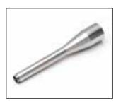
The RA0019 is an adapter for using a 1/4" microphone with a 1/2" preamplifier. Its influence on the acoustic field is minimal. To reduce attenuation of the microphone signal, the guard ring of the preamplifier is extended through the RA0019.
