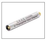
The RA0080 is a 6pF input adapter for 1/4" preamplifiers. One end screws on to a 1/4" preamplifier and the other end has a Microdot (UNF 10-32) input connector. This enables connecting a signal generator to the input of
