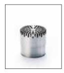
High precision microphone for laboratory work and coupler measurements (e.g. in the G.R.A.S. IEC 60318-1 (60318) Ear Simulator RA0039). Has a frequency range from 3.15 Hz to 20 kHz. Its size and low sensitivity makes it extremely robust and stable and can measure sound pressure levels up to 164 dB.
