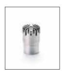
Low sensitivity microphone for high level and high frequency measurements. Its low sensitivity makes it ideal for measuring high sound pressure levels of up to 172 dB. Its small size reduces the effects of diffraction and reflections around the microphone, resulting in a frequency range reaching up to 100 kHz.
