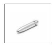
The RA0173 is a 1/8" nosecone for replacing the standard protection grid of a 1/8" microphone when making acoustic measurements in laminar airflow. The tip should be pointed upstream in a laminar
