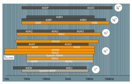
The Part or Model number of each microphone is also shown. The microphones are grouped according to size of external diameter, i.e. 1", 1/2", 1/4" and 1/8".
