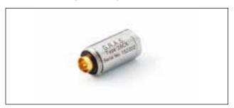
G.R.A.S. 26CK 1/2" Preamplifier is a very small preamplifier optimized for use with prepolarized condenser microphones. It is a robust unit that uses a constant current power (CCP) supply. The 26CK has a very low inherent noise level, a large dynamic range, and a frequency response from below 2 Hz to above 200 kHz.
