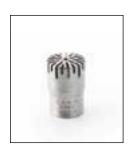
Low sensitivity microphone for high level and high frequency measurements. Requires no polarization voltage. Its low sensitivity makes it ideal for measuring high sound-pressure levels of up to 168 dB. Ideal with CCP preamplifiers and for sound measurements at very high frequencies and levels.
