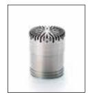
Low frequency microphone especially designed for infrasound measurements. Frequency range from 0.5 Hz to 20 kHz. Use the dedicated ¼" CCP preamplifier G.R.A.S. 26CG in order to obtain the low frequency response.
