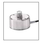
The microphone set 47DX is a low profile 1/8" precision pressure microphone with built-in CCP preamplifier. With a height (to the diaphragm) of only 9 mm, 47DX is suitably designed for flush mounting in plates in ground array applications and other applications with size constraints.
