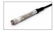
46BF is a 1/4" high frequency free-field microphone set for high level measurements with built-in TEDS and integrated 3 meter cable with a 7-pin LEMO connector.
