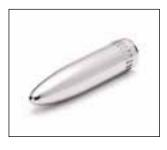
The RA0020 is a 1/2" nosecone for replacing the standard protection grid of a 1/2" microphone when making acoustic measurements in laminar airflow. The tip should be pointed upstream in a laminar
