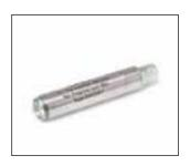
The RA0067 enables a prepolarized 1/2" microphone (typically a G.R.A.S. 40AD) to be used as a high impedance sound source. It takes a calibration signal directly from a signal generator. This makes the micro-
