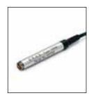
Similar to G.R.A.S. 26AC but with 40  $G\Omega$  input impedance to enable low level and low frequency noise measurements. 3 m cable with a 7-pin LEMO connector included.
