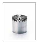
High precision microphone for laboratory work and as a working standard microphone in calibration laboratories. Wide frequency range from 3.15 Hz to 40 kHz. Its size and low sensitivity make it extremely robust and stable and can measure sound levels up to 164 dB.
