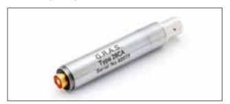
CCP preamplifier with integrated BNC connector. For use with 1/2" prepolarized microphones and standard constant-current input devices. Includes built-in TEDS which enables it to be programmed as a complete unit together with a microphone.
