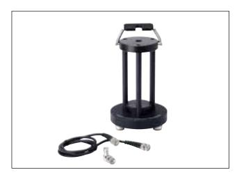
AL0011 provides a convenient platform for calibrating IEC 60318-1 Ear Simulators, e.g. G.R.A.S. RA0039. The stand and the adapters are designed for standardized frequency calibration using a transmitter setup with a microphone as sound source (not included) and the 14AA Electrostatic Actuator Amplifier for driving the setup.
