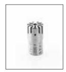
Low sensitivity microphone for sound measurements at high frequencies and high levels. Its low sensitivity makes it ideal for measuring high sound pressure levels of up to 175 dB. Its very small size reduces the effects of diffraction and reflections around the microphone, resulting in a frequency range extending up to 80 kHz.
