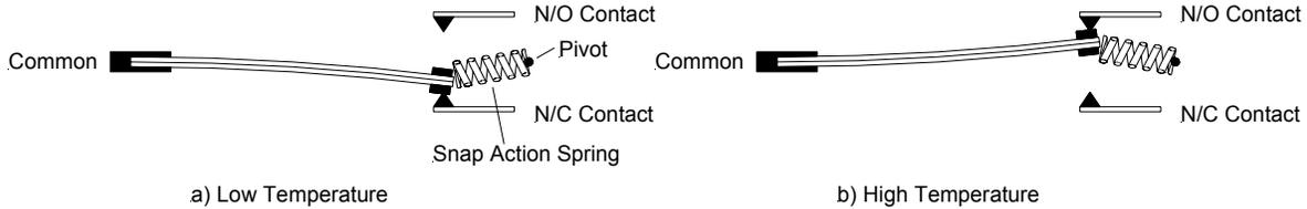
**Figure 9-2 - Bi-metallic Temperature Switch with Snap Action**
