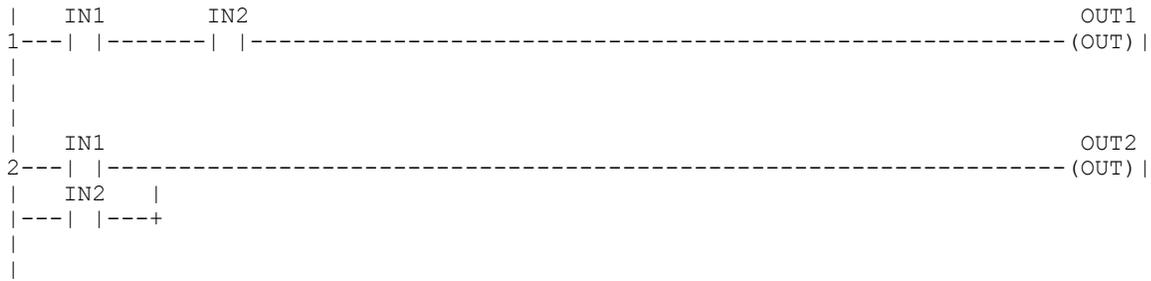
**Figure 3-6 - PLC Program with Added OR Rung**
