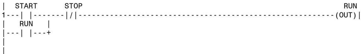
**Figure 12-4 - Improved Start/Stop Program With Overriding STOP**
